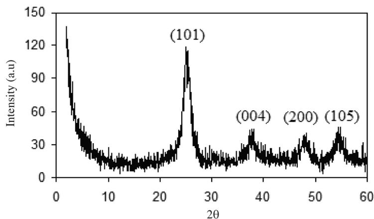
FIGURE 3. XRD pattern of TiO<sub>2</sub> anatase phase which have intensity at peak (101), (004), (200) and (105)
