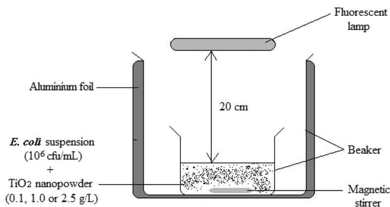
FIGURE 1. Experimental setup for photocatalysis reaction under fluorescent lamp
