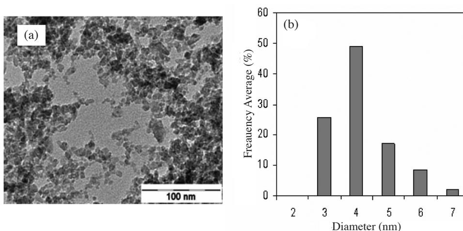
FIGURE 2. (a) Transmission electron micrograph (TEM) image of TiO<sub>2</sub> nanoparticles powder heated at 100°C and (b) distribution size of TiO<sub>2</sub> nanoparticles
