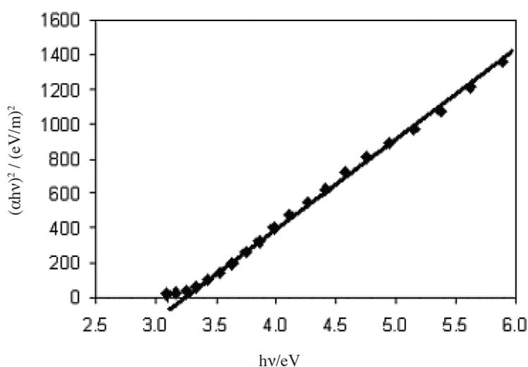
FIGURE 5. Extrapolation of graph  $(\alpha h\nu)^2$  vs  $h\nu$  for TiO<sub>2</sub> nanoparticles with 3.2 eV band gap energy
