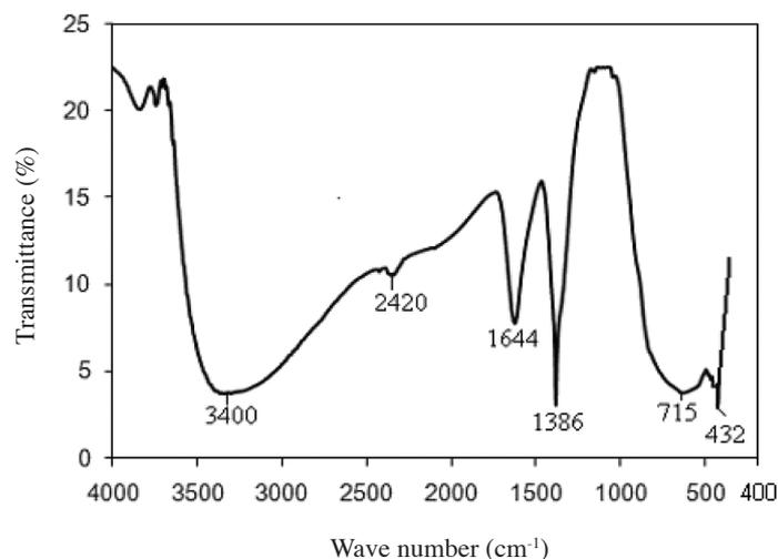
FIGURE 4. FTIR spectrum of TiO<sub>2</sub> sample
