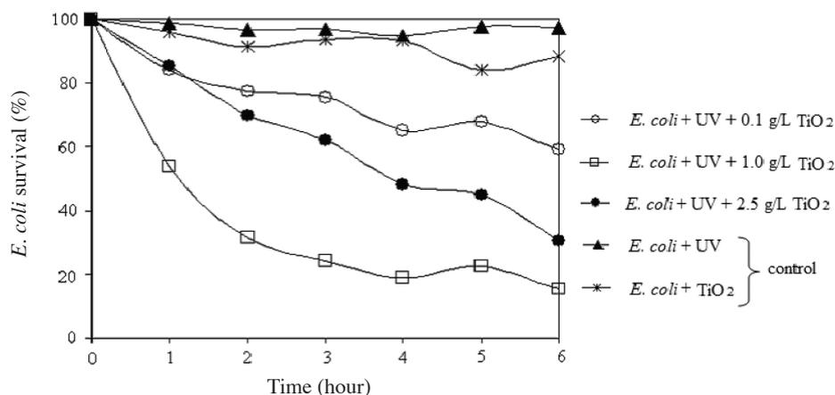
FIGURE 6. The effect of TiO<sub>2</sub> nanoparticles towards survival of *E. coli* during photocatalytic process
